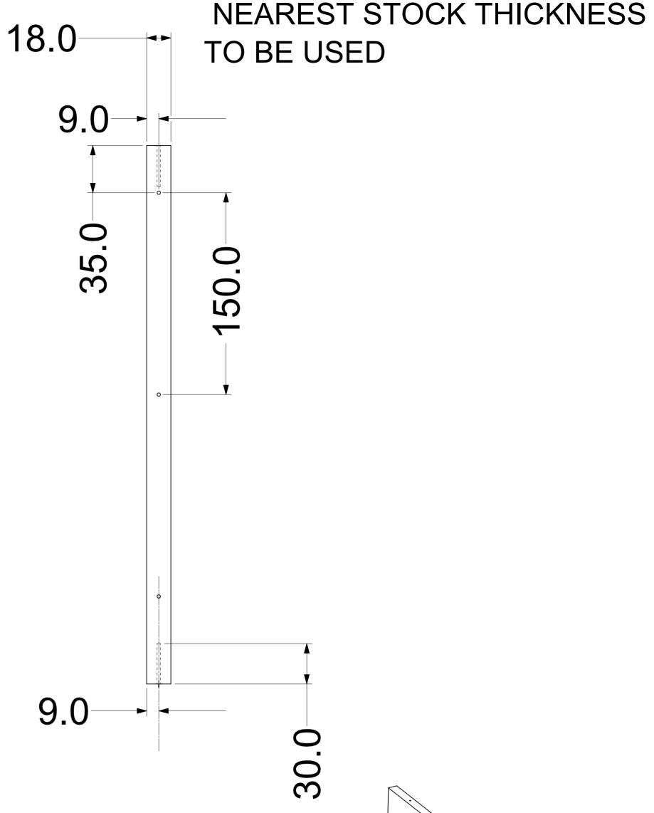
DETAIL NO. RAD0005 ELECTRICAL COMPARTMENT BACK PANEL
