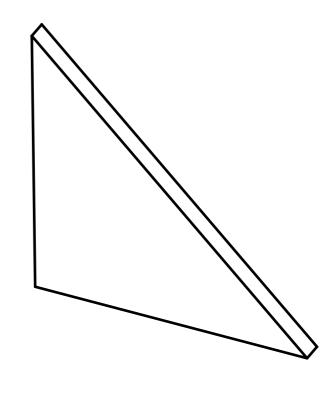
DETAIL NO. RAD0045 GUSSETT FOR MOTOR MOUNTING BRACKET
