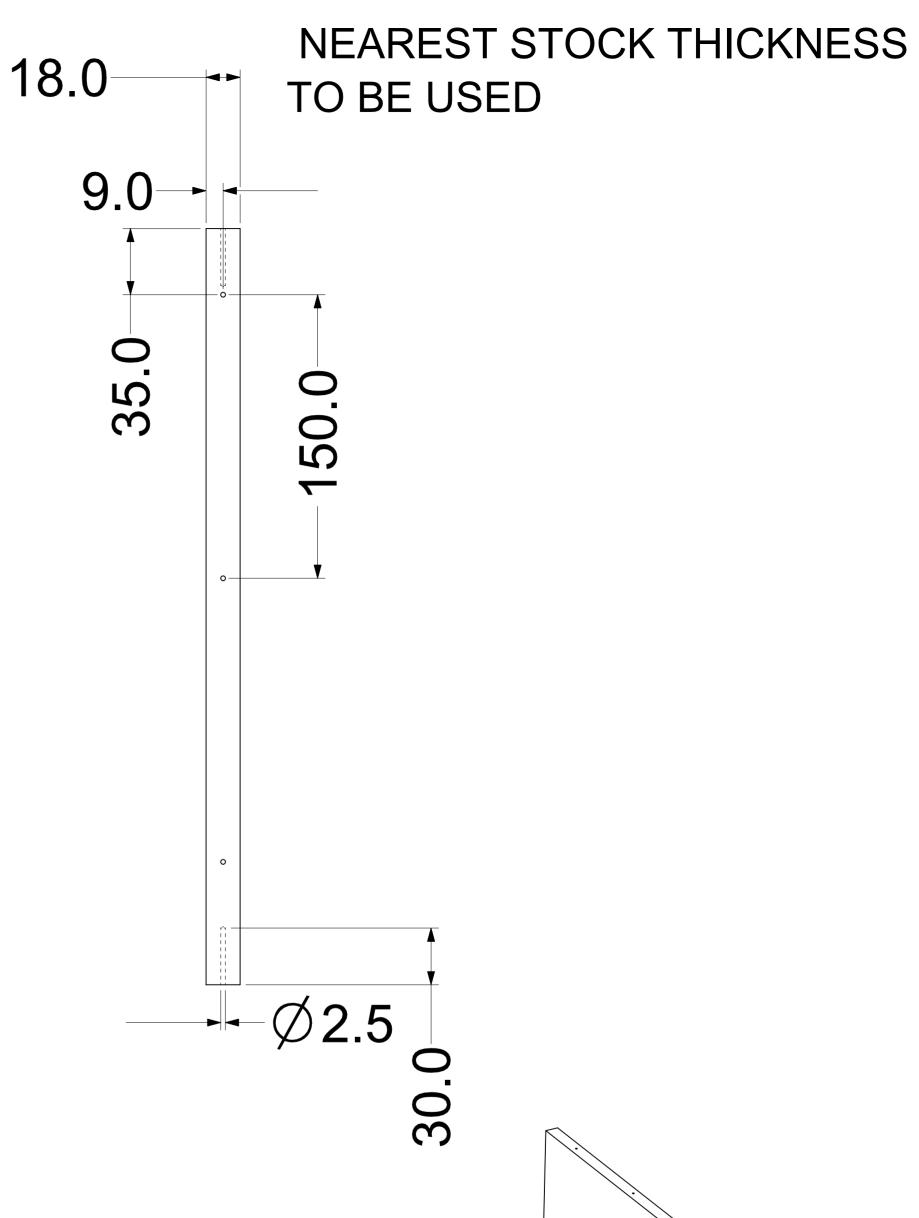
DETAIL NO. RAD0005 ELECTRICAL COMPARTMENT BACK PANEL
